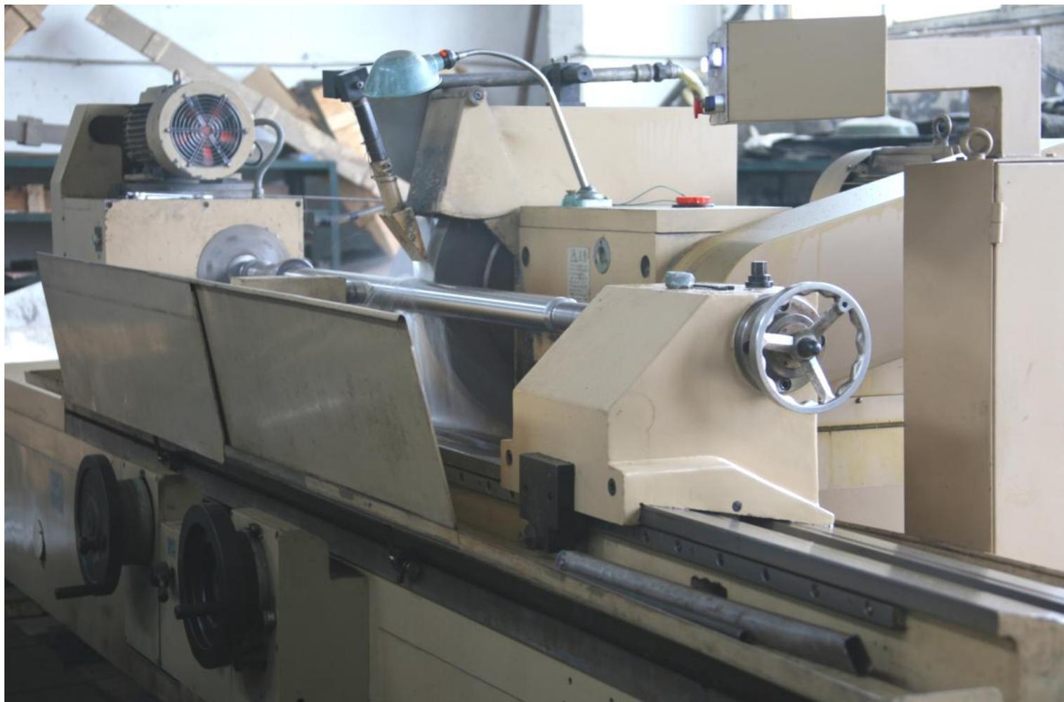
主轴外圆磨床 Cylindrical grinder for main shaft
